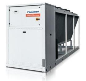
Air-Source Heat Pumps for outdoor installation, for the production of chilled or hot water. The units feature hermetic scroll compressors using R-410A refrigerant, axial fans, plate heat exchanger, condensing coils with copper tubes and aluminum fins and electronic expansion valve. The range is composed by units equipped with two compressors in a single-circuit configuration.
