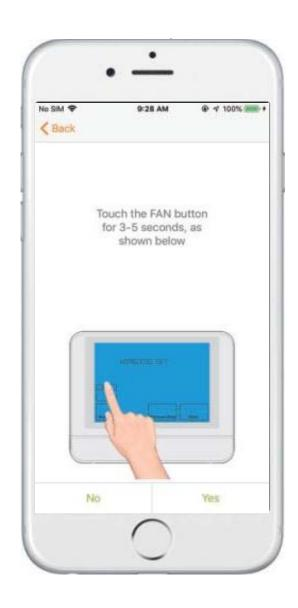
Step 5 - Thermostat enters the binding state
